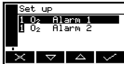
Figure 19 - The Alarm set up screen
