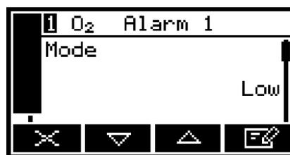
Figure 20 - The Alarm mode screen
