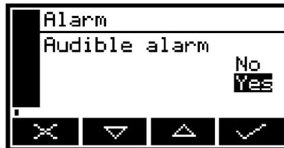
Figure 21 - The Audible alarm option screen
