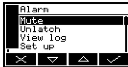
Figure 18 - The Alarm option screen
