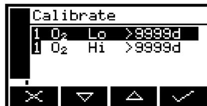
Figure 16 - The Calibrate screen
