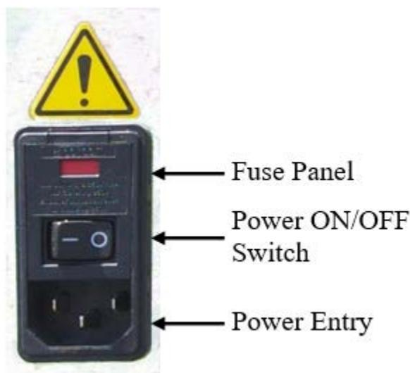
*AC Power Switch, Connector and Fuse.*
