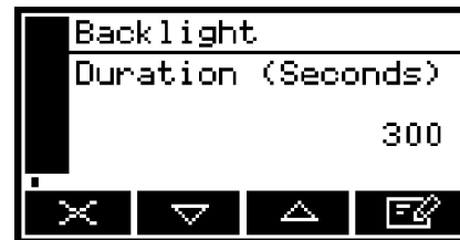
Figure 22 – The backlight timer screen
