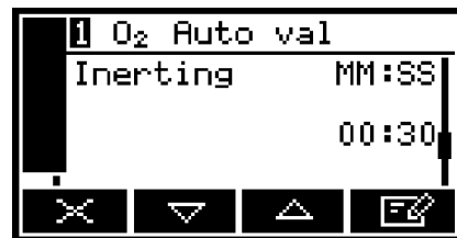
Figure 40 – The auto val/cal inerting timer screen
