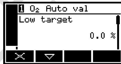
Figure 30 – The auto val/cal low target value screen
