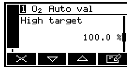
Figure 32 – The auto val/cal high target value screen
