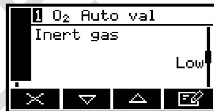
Figure 39 – The auto val/cal inert gas screen
