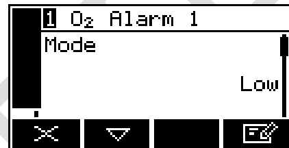
Figure 58 – The alarm mode screen
