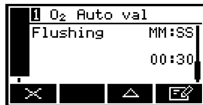
Figure 41 – The auto val/cal flushing screen
