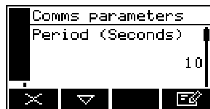
Figure A2 – The serial output period screen
