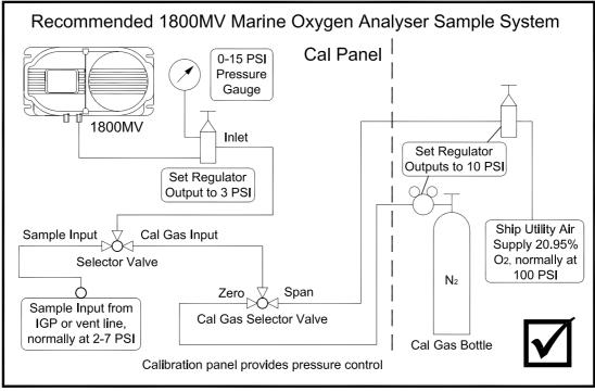
Figure 1 Installation Schematic
