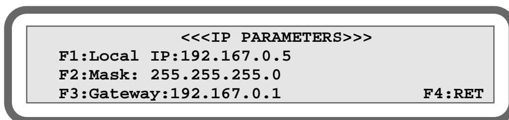
**FIGURE 30: IP PARAMETERS**
