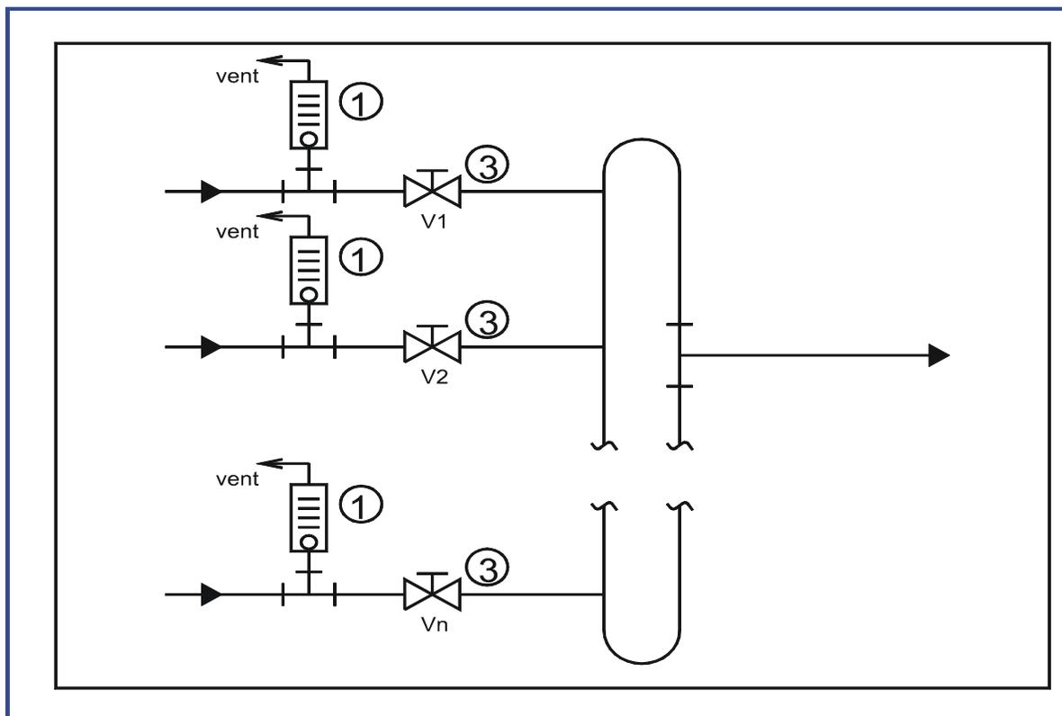
The loop eliminates the problem introduced by the length of section ④. Here only dead volume introduced by section ③ is present. By making these lengths as small as possible, the problem still is tolerable.
