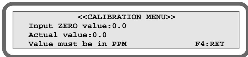
**FIGURE 5: DISPLAYED WHEN ENTERING ZERO VALUE**
