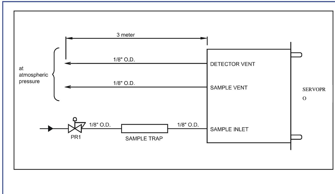
PR1 is a miniature stainless steel high purity pressure regulator. The internal volume must absolutely be at its minimum. Any unswept dead volume will cause noise and instability and, will cause poor recovery time. PR1 should be installed close to the sample point. PR1 should be installed only if there is large pressure excursion (over 69 kPa (10 PSIG)).
