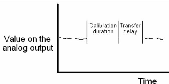
FIG 8: TRANSFER DELAY
