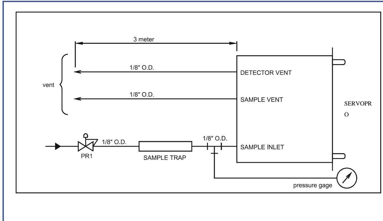
Some users wish to monitor the inlet pressure. Connecting a pressure gauge at the inlet will result in big unswept volume. This will cause poor response time, drift and noise. **DON'T DO THIS!**
