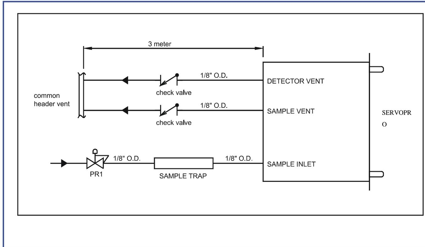
Some users wish to avoid back flow from a vent header into the analyzer vent. Doing so will cause sample flow and cell pressure variation. The cell pressure will follow header pressure variation. Check valve cracking pressure is not constant. The plasma cell must work at atmospheric pressure with no backdraft. Problems caused:
