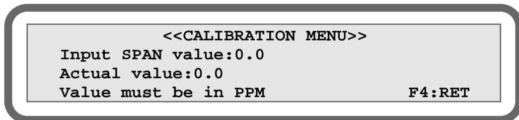
**FIGURE 6: DISPLAYED WHEN ENTERING SPAN VALUE**
