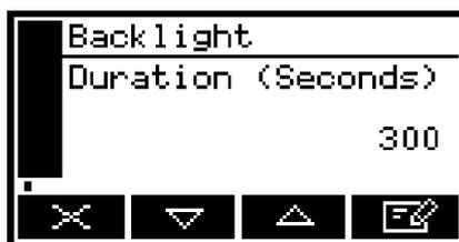
Figure 39 - The Backlight timer screen
