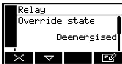
Figure 37 - Relay override state screen
