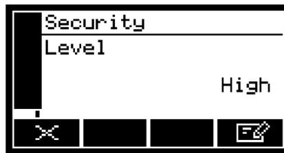
Figure 14 - The Security level screen
