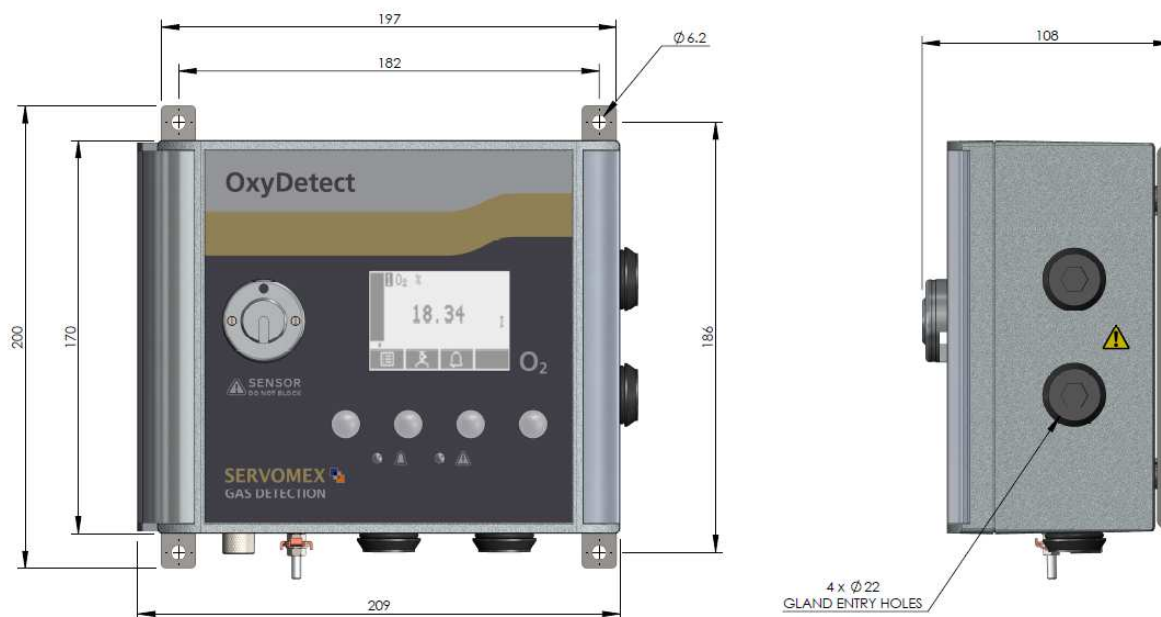
Figure 11 - OxyDetect dimensions (in millimeters)
